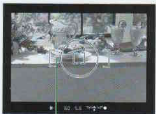
Partial metering circle.
